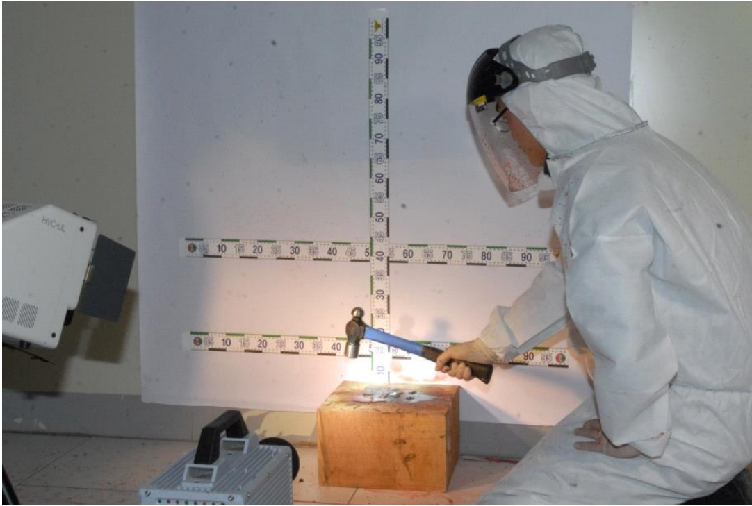
(An experiment on velocity measurement of the impact spatters by a hammer (2011))
