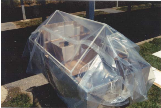
Greenhouse to conduct hot range temperature experiments.
