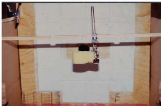
Tile for high velocity experiment in a specially constructed chamber.
