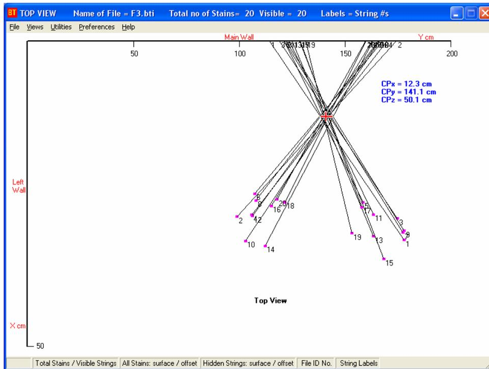
*Figure 1a. Top view of Pattern #18. The average position for the line-crossings corresponds to the X- and Y-coordinates of the blood source location, in the plane of the floor.*
